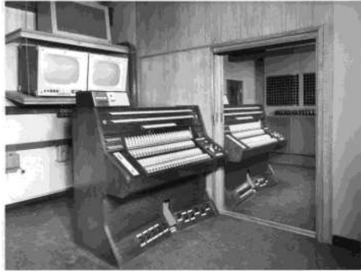
Two Strand SYSTEM CD TV Light Consoles with conventional Compton hardware and memory pre-sets, in adjacent BBC Television installations, Wembley Studio 5, UK.
