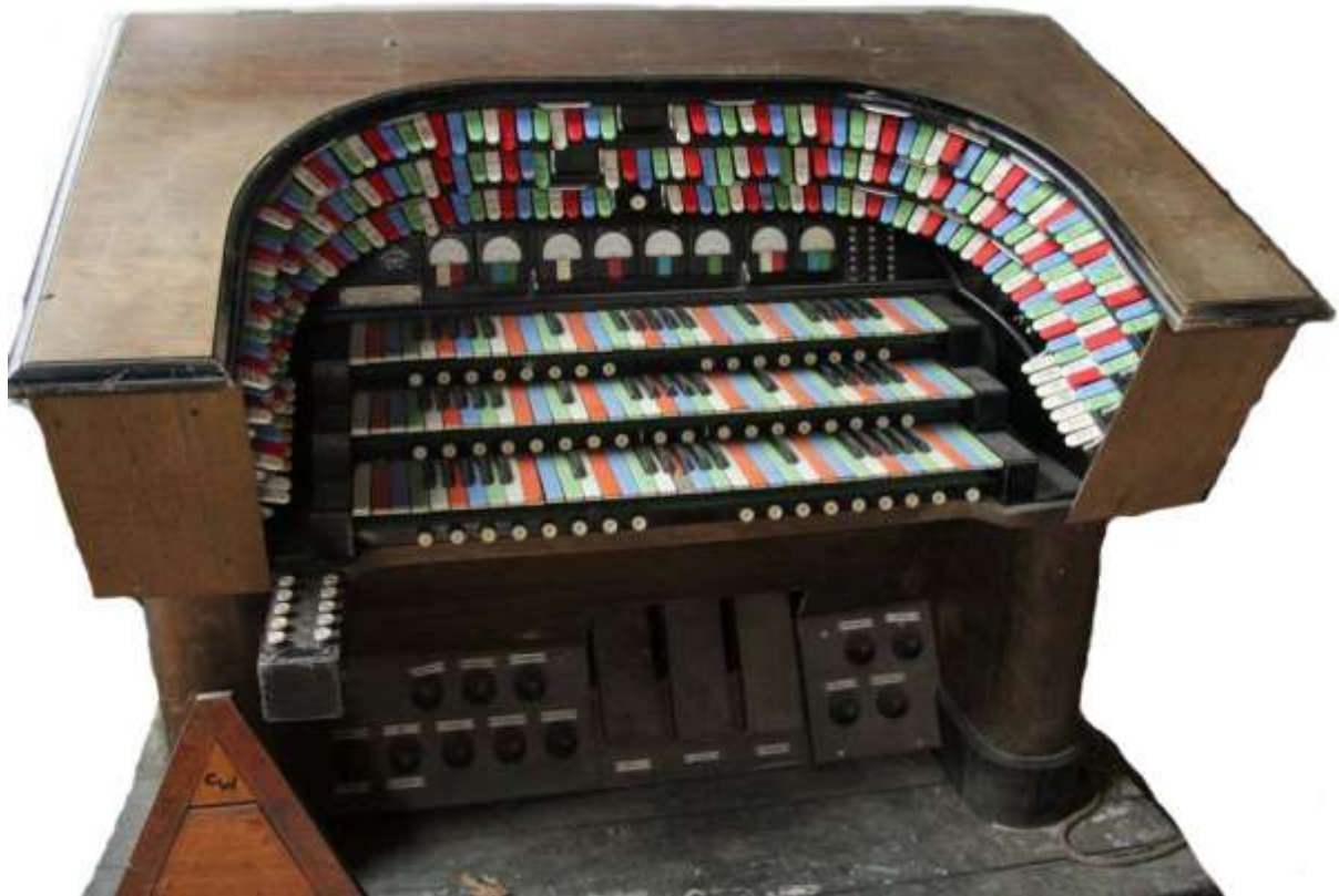
The COMPTON Built / STRAND Light Console along with all its 1929 organ technology installed in the Theatre Royal, Drury Lane, London, UK in 1950.
